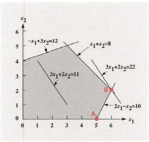
Using the primal simplex method, one can pivot from the vertex labeled A to the vertex labeled B. Consider this pivot.
