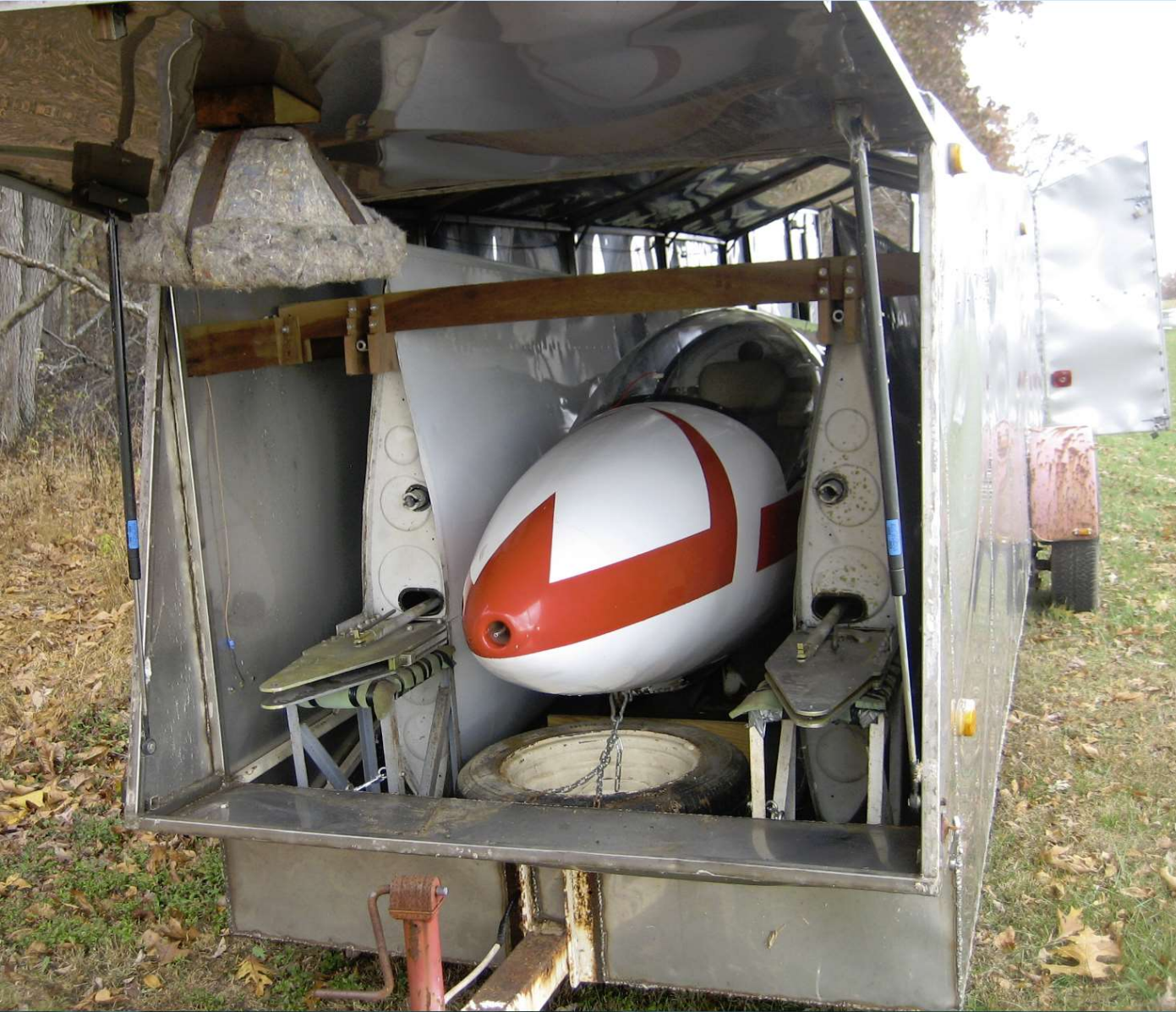
Front of Ship in the Stainless Steel Closed Trailer – Note Cushioned Nose Cone and Spare Tire
