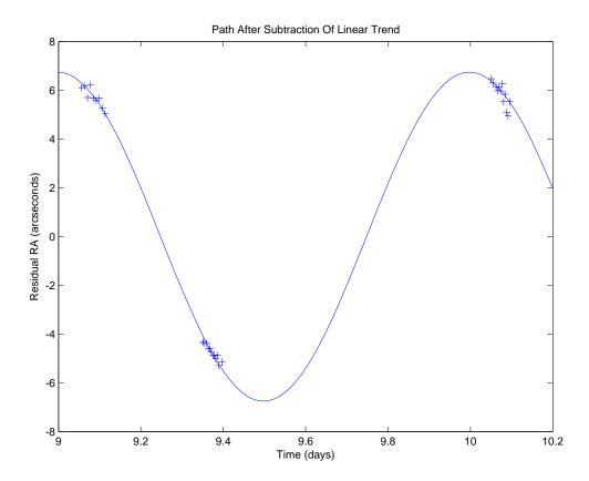
Fig. 2.— After the uniform linear motion due to the Earth's and Prudentia's solar orbits is subtracted out, the residual shows the sinusoidal RA motion of Prudentia across the sky due solely to the rotation of the Earth.
