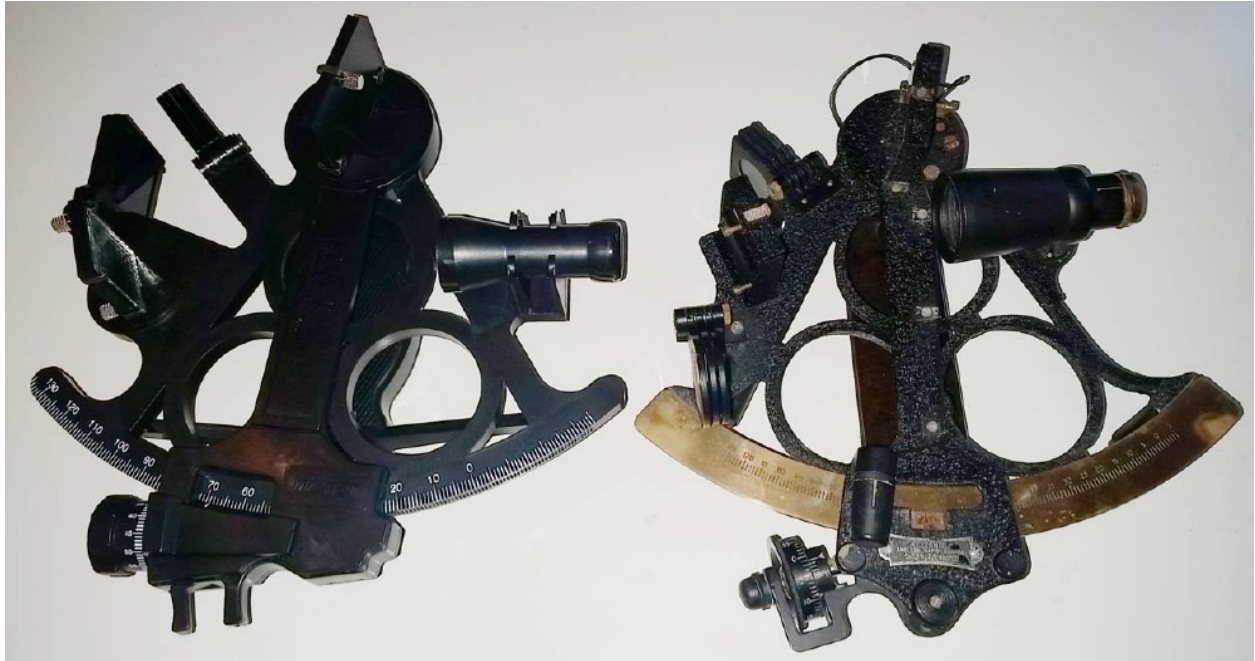
Figure 2 The two sextants used to make the measurements. The plastic sextant is on the left and the “real” one, a second-hand professional sextant from the 1970s, is on the right.
